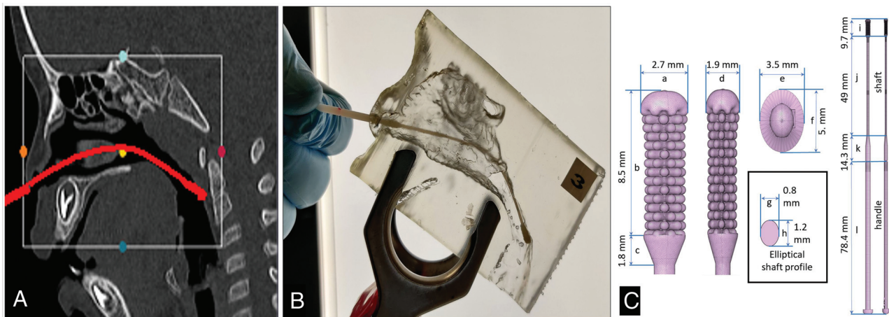
FIG 1. A, Sagittal section of a maxillofacial CT scan of a 22-month-old patient. Shown in red is the trajectory of a virtually inserted swab reaching the posterior nasopharynx. The white box shows the portion of the anatomy chosen to print the nasopharyngeal passage. B, A commercial flocked pediatric swab (COPAN Flock Technologies swab) reaching the posterior nasopharynx within the 3D-printed nasopharyngeal passage. C, Design of the elliptical-section 3D-printed pediatric swab (Design ES).
